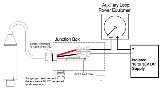
Connect Red conductor to +ve supply Connect Black conductor to -ve supply.
