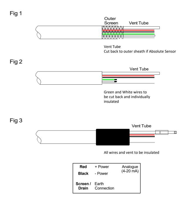
Cable is normally provided to the required length with the ends terminated as depicted above.
