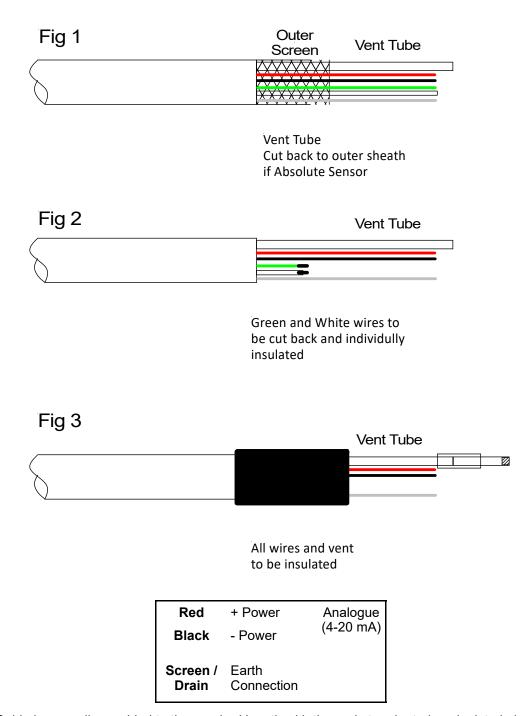
Cable is normally provided to the required length with the ends terminated as depicted above.
