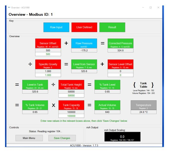
This screen provides an overview of the APT1000 calculation chain, the current configuration values set, and the calculated results. These are detailed as follows:-
