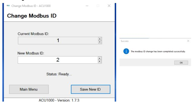
This screen displays current Ident number of the connected APT1000 and allows entry of a new one. Once desired Ident is selected press Save New ID to write to the APT1000. and allow the process to complete before quitting to main menu. A confirmation message is shown.
