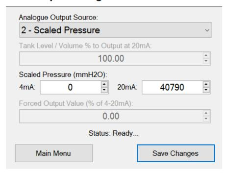
This screen allows which parameter the mA output represents to be selected from the drop down menu.
