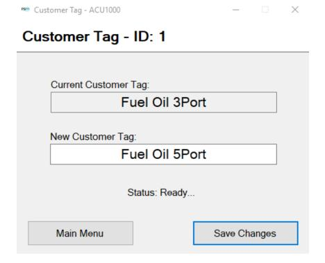
This screen reads the current tag when opened and displays it in the "Current Customer Tag" box. A new Tag may be typed in and written to the APT1000 by using the "Save Changes" button. Note that the Tag may have a maximum of 20 characters including spaces.
