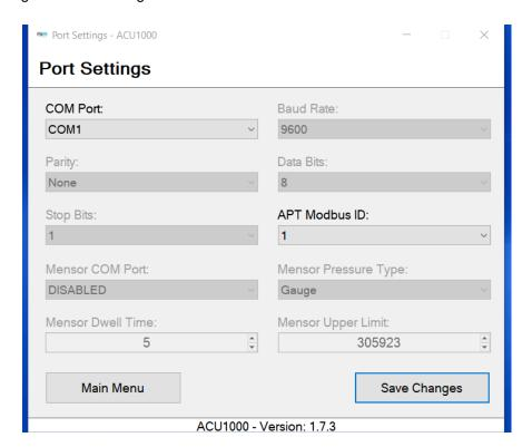
In the COM Port Field use the drop down to select the Com Port that Windows has assigned to the USB to RS485 converter (as described previously using Device Manager).
