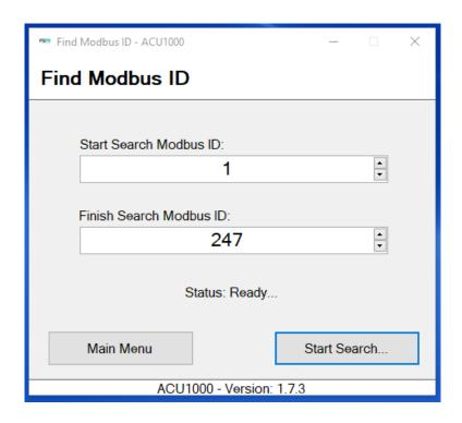
The utility sequentially searches for Ident numbers in the range between the start and finish ID numbers entered. Note that 247 is the maximum ID value.
