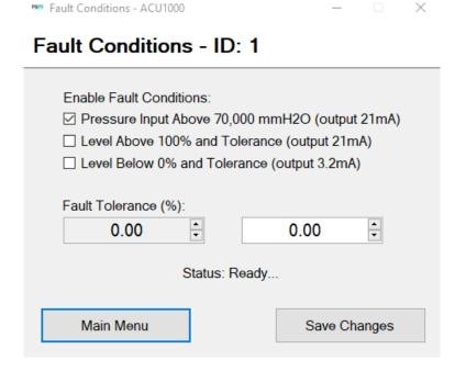
This screen allows selection of the conditions which will cause the mA output to drive to its fault indication current value of either 3.2mA or 21mA,
