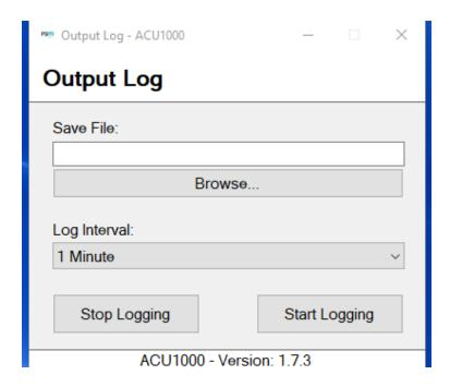
This screen enables the pressure and temperature values to be logged to a CSV file.
