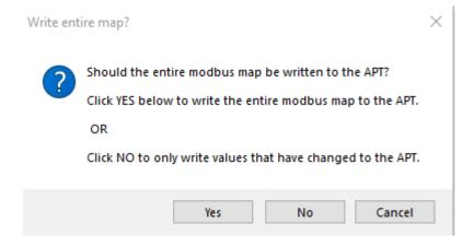
Once the selection is made the appropriate write action is taken. A status message above the control buttons indicates progress and success.
