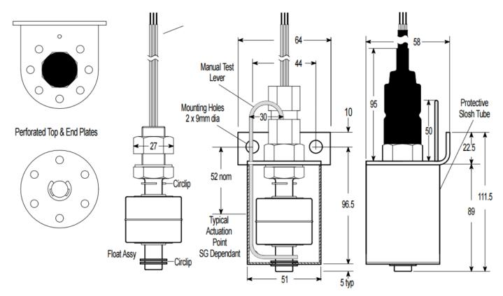
The nominal switch actuation point is at a dimension of 50mm below the mounting holes and actuates on a rising level, therefore in tank fixing should be located at a datum of 50mm above the desired alarm actuation point.
